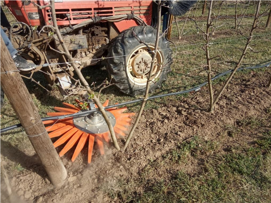
Tree-row management with rolling cultivator + finger weeder (mechanical weed control and SF incorporation)
